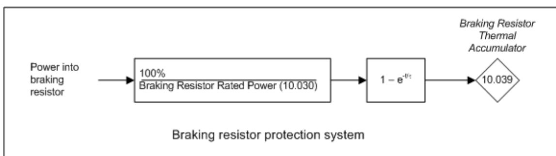
The drive monitors the power flowing into the braking resistor and updates the *Braking Resistor Thermal Accumulator* (10.039). If bit 1 of *Action On Trip Detection* (10.037) = 0 and the accumulator reaches 100% an *Brake R Too Hot* trip is initiated. If bit 1 of *Action On Trip Detection* (10.037) = 1 and the accumulator reaches 100% the braking IGBT is disabled until the accumulator falls below 95.0%.
