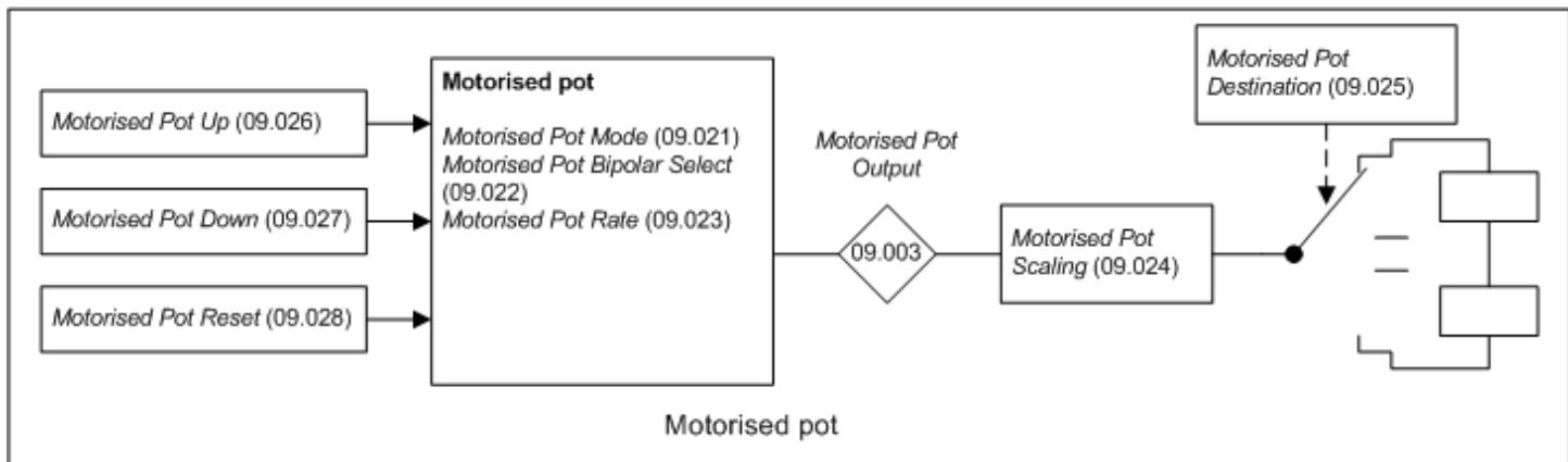
If *Motorised Pot Reset* (09.028) = 1 then the motorised pot is disabled and held in its reset state with *Motorised Pot Output* (09.003) = 0.0%. If *Motorised Pot Reset* (09.028) = 0 the motorised pot is enabled even if *Motorised Pot Destination* (09.025) is not routed to a valid parameter. The sample rate of the motorised pot is always 4ms.
